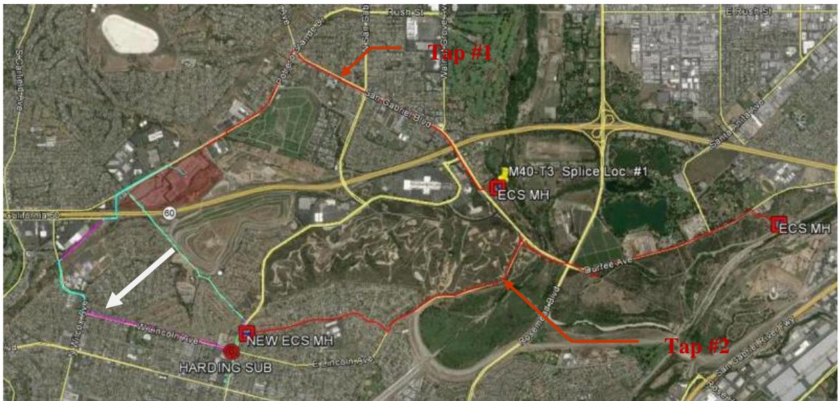
An existing overhead cable route that runs southeast from Mesa Substation to Harding Substation will be removed from existing poles and installed on existing poles (pink) and existing underground conduit (turquoise) as indicated by the white arrow in Figure 4-3. The fiber optic cable will be reinstalled to existing conditions following the completion of the Mesa substation build out.
